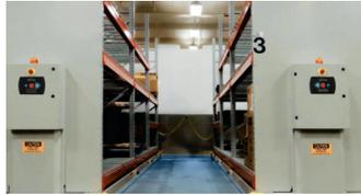
Photoelectric beams projecting on both sides of each aisle are mounted low on the carriage side members.
