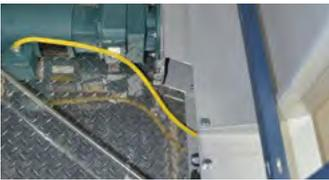
All mechanical moving components are concealed and protected by a steel safety guard to prevent inadvertent access.
